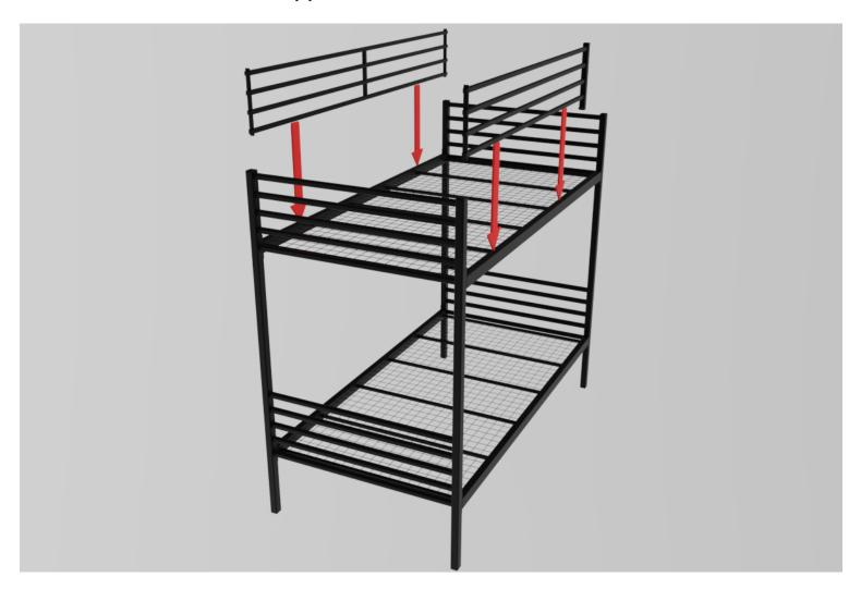
Attach front and back safety rails to frame by the relevant bolt holes.
